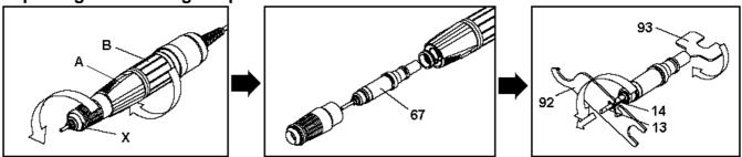
To remove or replace the pliers 14, follow the operating sequence and comply with the procedure by help of the above pictures (work with the sample test bur inserted - 13).
